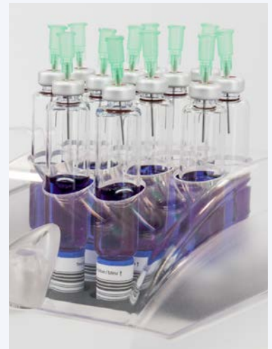
Oxidation of organic carbon compounds contained in the sample to CO 2
